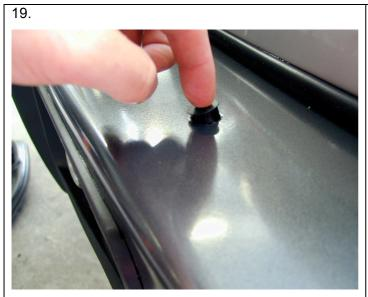
There are two Ø16 holes located on the top face of the bar. If no CB aerials are fitted the holes can be covered with the plastic plugs provided in the fitting kit.
