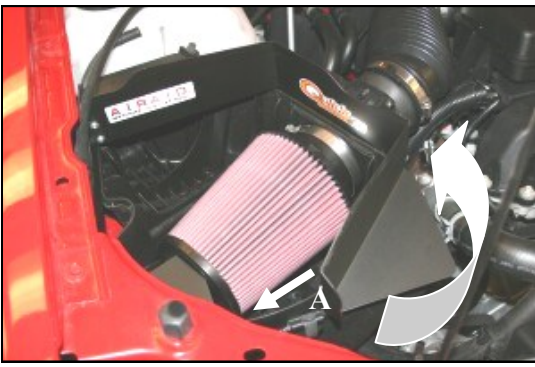
6. Install the Quick Fit panels by inserting the tab on the front of the panel into the front slot of the factory airbox base (A), and then rotating the panels counterclockwise.
