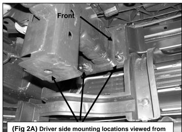
(Fig 2A) Driver side mounting locations viewed from behind the bumper (non tow hook equipped models)
