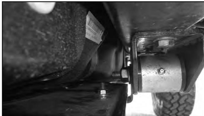
26. Mark the hole location for the skid plate support bracket on the bottom of the fuel tank skid plate.
