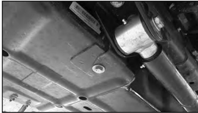
29. Torque the 9/16" hardware for the Recoil Traction Bar at the frame and axle brackets to 90 ft-lbs.
