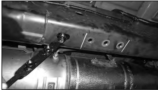
24. Attach the frame bracket to the frame rail with three of the 1/2" x 1-1/2" bolts and 1/2" SAE washers from Bolt Pack 963. Torque the 1/2" bolts to 60 ft-lbs.
