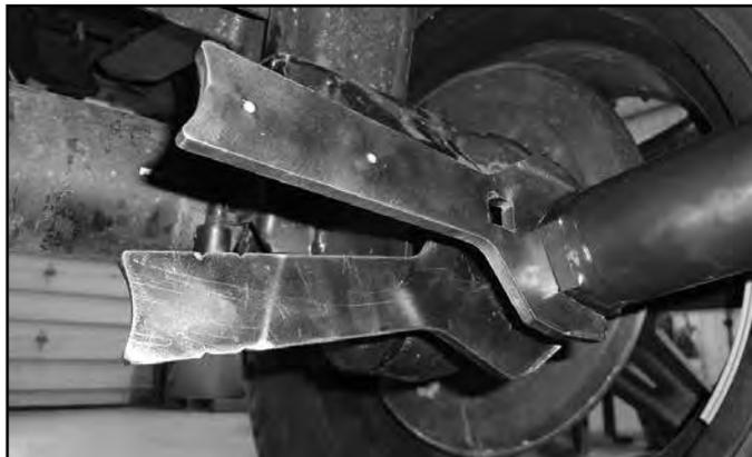
35. Use the levels on the wrench to gauge how much force is inputted into the Recoil Traction Bar. The wrench is designed to be used at the traction bar slider end as shown in Figure 23. Make sure the wrench is pressed firmly against the bushing / tube for an accurate measurement.
