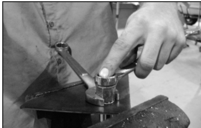
FIGURE 2 - 1/2" RIVET NUT SHOWN
