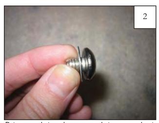
Put one pocket washer on a pocket screw and put screw through a pocket hole in the flare, screw head on the outside.
