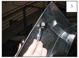
Place a pocket nyloc nut over the end of the screw and tighten, using a 1/2" wrench for the nut and the supplied T45 torx bit for the screw.
