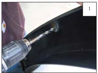
Using the indents in the flare pockets as a guide, drill a 5/16" hole from the backside.
