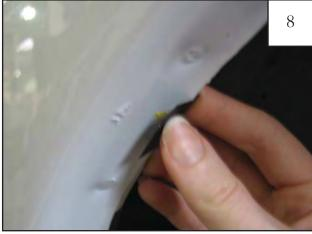
Install plastic tab on sheet metal centered over mark.
