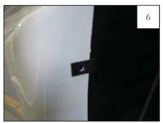
Install narrow clip over existing factory hole.
