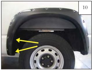
Hold flare in place on vehicle and start #8 pan-head screws through holes in flare, narrow clips, and into factory holes using a #2 Phillips screw driver. *Do not tighten*.
