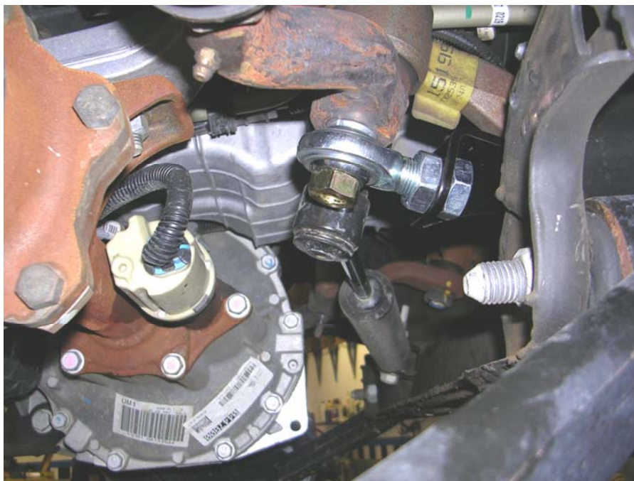
Figure 3: idler arm bracket installed
