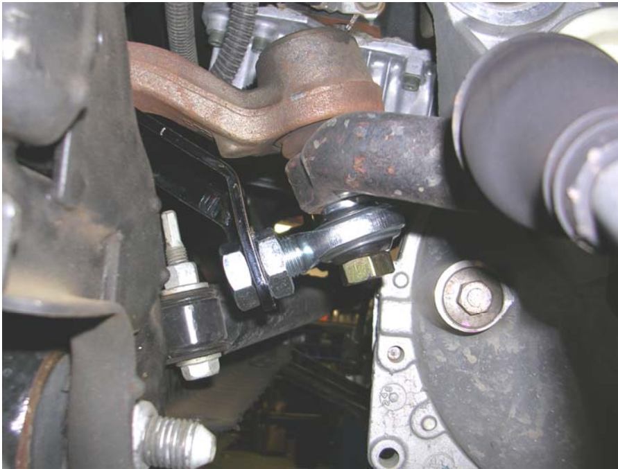
Figure 5: pitman arm bracket installed
