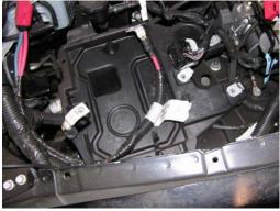
11. Remove the three nuts (1) securing the battery tray (2) to left inner fender (3). Lift the battery tray (2) out of the engine compartment and remove from the vehicle.
