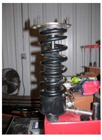
31. Reinstall the strut assembly into the vehicle and start the upper nuts, hand tighten only. Reinstall the lower strut clevis and hand tighten the bolt at the strut. Install the lower clevis bolt into the lower control arm.
