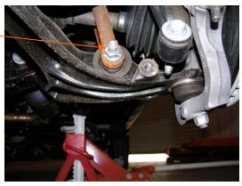
20. Remove the upper control arm ball joint nut with a 21mm wrench and separate the upper ball joint from the knuckle.
