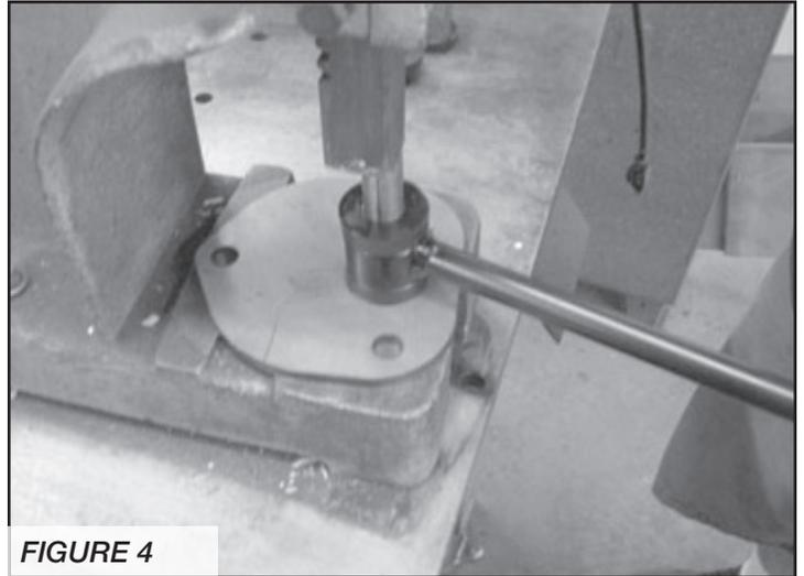
5. Using a 1/2" drill bit, drill out the sway bar to 1/2". **SEE FIGURE 5**
