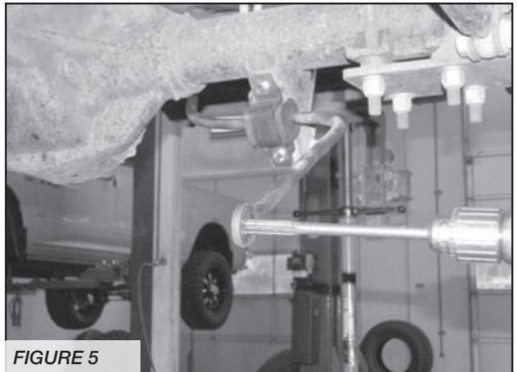
6. Locate the FT30475 nut tab, one 1/2"-13 x 2-1/2" bolt and a 1/2" washer. Mount the link to the frame using the hardware listed above. Torque to 90ft-lbs.
