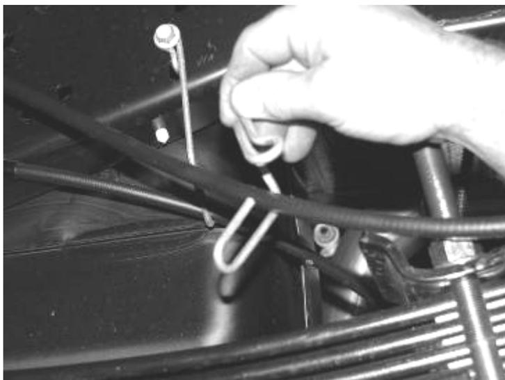
3. Locate and install the rear lift blocks, the factory block will be positioned on top of the new Fabtech block, with the short center pin of both blocks facing down, to the axle. The short end of the blocks should face to the front of the vehicle. Using the supplied u-bolts, nuts, and washers align axle, lift blocks, and springs and torque to U-Bolts to 90lbs. SEE PHOTO BELOW
