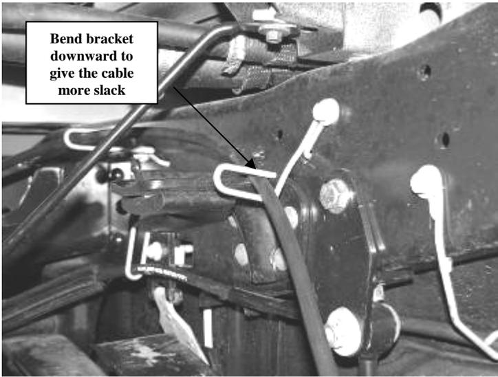
axle using the factory hardware. Using the supplied 3/8" x 2" bolt, nut, and washer attach the brake line to the other end. Reattach vent line. SEE PHOTO BELOW.
