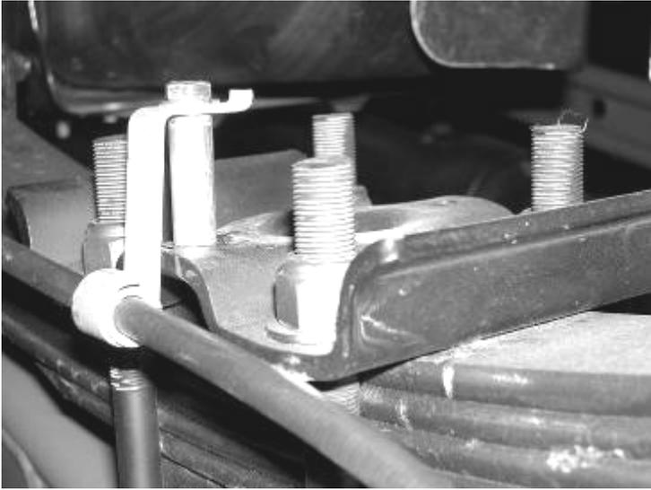
9. Install Fabtech shock part number FTS7266 Performance Shocks or FTS81005 Dirt Logic (not included) with the factory hardware and torque bolts to 65ftlbs.
