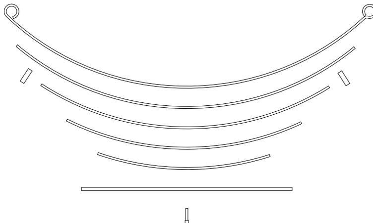
4. Realign the center pin in the leaf spring pack to the centering hole on the axle perch and install the original u-bolts. Torque u-bolts to manufacture specifications.
