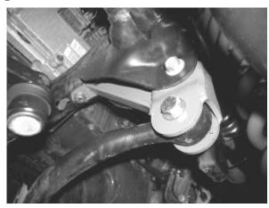
16. Connect the drag link to the new drop pitman arm. Torque the original nut to 45 ft/lbs. SEE PHOTO BELOW.
