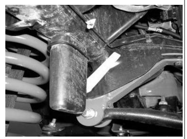
10. Locate FT44103 upper link arms. (**This link is 18" from the center of the barrel to the center of the barrel**). Press one FT1037 small bushing and one large FT1038 bushing
