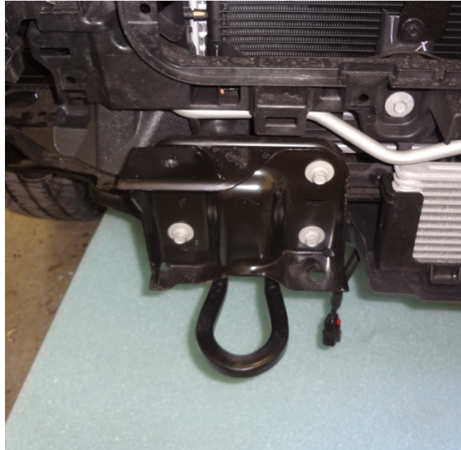
Figure 3b (TOW HOOK & OEM MOUNTING BRACKET)
