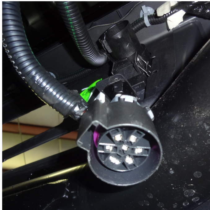
Figure 3a (ELECTRICAL HARNESS DISCONNECTED)
