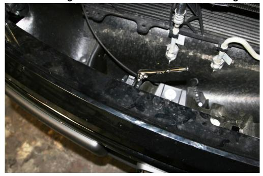
E. Remove 5 plastic tree clips holding the rubber dust
