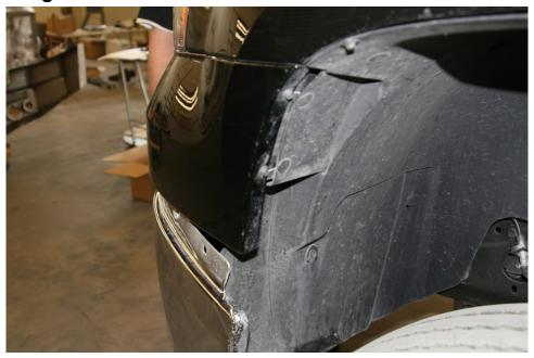
D. Reaching behind the grill use needle nose pliers or a flat bladed screwdriver to pop loose all clips holding the painted bumper section to the grill.
