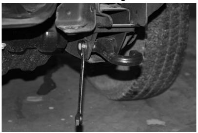
L. Remove the two plastic brackets at the front of each fender by removing the two dart clips from the wheel well and the three 10mm bolts. See Image Below
