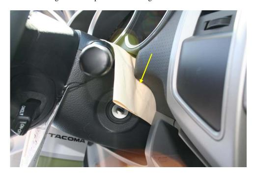
iii. Starting on the left-hand side, gently separate the upper Instrument Panel Bezel.1. Rotate it up and to the left and let it hang.
