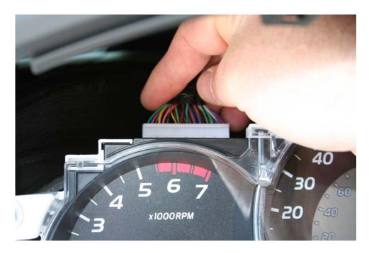
f. Using the supplied cable, connect the small black connector (C3) to the VSS inline module.
