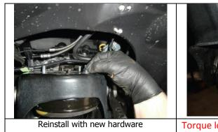
Reinstall/torque wheels/tires and
