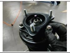
Install new strut extension with OE hardware and tighten.
