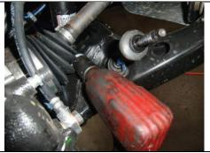
. Disconnect and remove lower shock bolt and nut.
