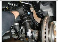
Remove strut assembly from vehicle
