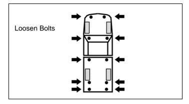
b. Remove body mount bolts from passenger side of vehicle ONLY.
