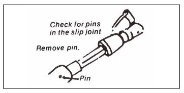
If your vehicle has no slip joint, an adjustment is necessary. Loosen adjusting nuts and bolts found on steering column under the dash near the firewall.
