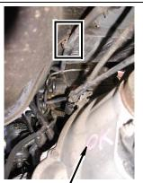
Body Clip Clutch Fluid Line (Inside of Wire Loom)
