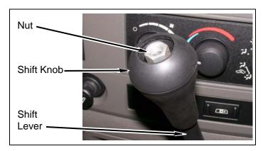
Remove transfer case shift lever boot from center console.
