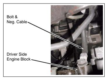
b. Install *kit* **bracket** (angled) onto engine with bolt. DO NOT TIGHTEN.
