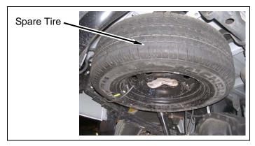
b. Remove retaining clip and ratchet tube from spare tire winch mechanism.
