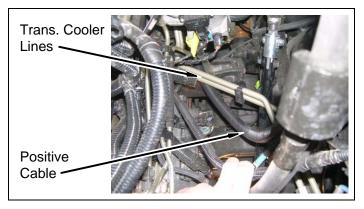
f. Route driver side positive battery cable behind transmission cooler lines. Install cable to transmission cooler lines with two *kit* ties (zip).
