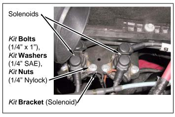
o. Install wiring harness push clip on *kit* **bracket** (solenoid).
