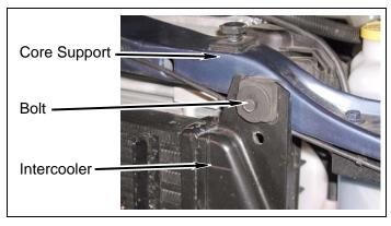
d. Push bottom of intercooler forward toward front bumper and remove two double bolt fasteners and front bumper from vehicle.
