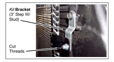
c. Install two *kit* brackets (3") onto two lower AC condenser mounts with two *kit* bolts (1/4" x 3/4"), four *kit* washers (1/4" SAE), and two *kit* nuts (1/4" Nylock). Ensure heads of *kit* bolts are facing forward. DO NOT TIGHTEN.
