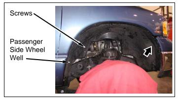
v. Install brake sensor wiring harness push clips onto passenger and driver side wheel wells.
