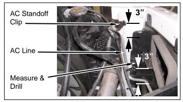
f. Drill two 1/4" holes into core support at marked locations and install two AC standoff clips.
