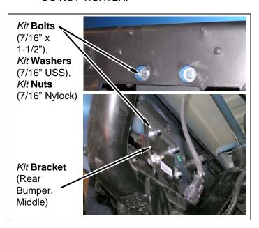
e. Install kit brackets (rear bumper) onto bumper with two factory bolts and u-nuts. DO NOT TIGHTEN.
