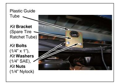
i. Install ratchet tube onto spare tire winch with retaining clip.
