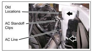
g. If removed, re-install AC condenser onto intercooler, and install AC line onto two AC line standoff clips. TIGHTEN all hardware.
