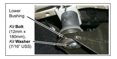
d. **2006 Models:** Remove each *kit* **bolt**, one at a time, and apply small amount of *kit* **Loctite**® onto threads. Install *kit* **bolt**, and captive washer. TIGHTEN *kit* **bolts** to **55** ft. lbs.
