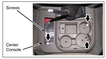
Install transfer case shift lever boot onto center console.
