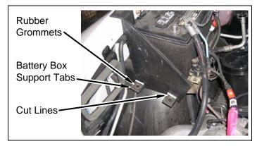
d. Mark two cut lines on battery box support tabs. Cut support tabs from battery box along lines. Where support tabs were cut from battery box, ensure smooth surface. Grind or sand, if necessary.
