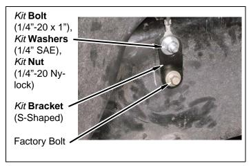
b. Install ground strap to *kit* **bracket** (S-shaped) with *kit* **bolt** (1/4"-20 x 1"), two *kit* **washers** (1/4"-20 x 1") and *kit* **nut** (1/4"-20 Nylock).
