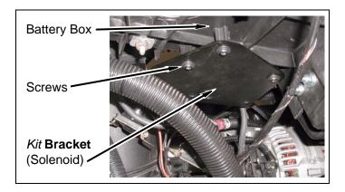
n. Install two solenoids onto *kit* **bracket** (solenoid) with four *kit* **bolts** (1/4" x 1"), eight *kit* **washers** (1/4" SAE), and four *kit* **nuts** (1/4" Nylock).
