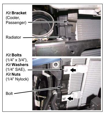
d. Install transmission cooler onto two kit brackets (cooler) with four kit bolts (1/4" x 3/4"), eight kit washers (1/4" SAE), and four kit nuts (1/4" Nylock).
