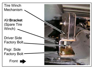
c. Install spare tire winch through hole in crossmember. Position spare tire winch onto *kit* **bracket** (spare tire winch). d. Turn *kit* **bracket** (spare tire winch) toward front of vehicle and slide spare tire winch cable through slot in *kit* **bracket** (spare tire winch).
