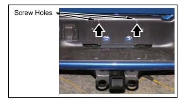
Remove two bolts from bumper bracket and bed.
