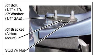
q. Install airbox onto *kit* brackets (airbox) and *kit* bracket (airbox mount) with *kit* bolt (1/4" x 1"), two *kit* washers (1/4" SAE), and *kit* nut (1/4" Nylock). TIGHTEN all hardware.
