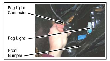
Remove four nuts from two double bolt fasteners.
