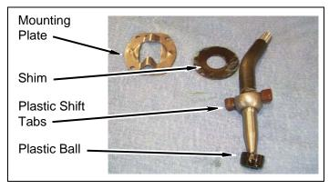
Scribe a line along side of transmission shift lever (below lowest bend). Measure diameter of shift lever (below lowest bend). Cut lever into two pieces and deburr as necessary.
