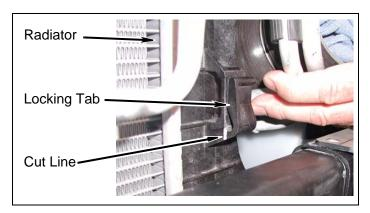
b. Cut two transmission cooler locking tabs flush along cut lines.
