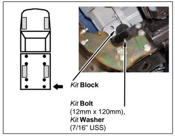
Install kit blocks onto two (or three) other frame mounts.
