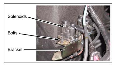
Remove three screws, wiring harness, push clip, and bracket from underneath passenger side battery box.
