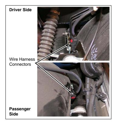
4. Remove two push clips and block heater cord from passenger side frame, if equipped.
