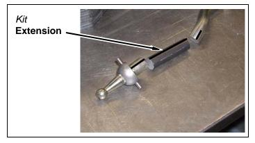
d. Grind welded surfaces smooth in order to install mounting plate and shim to shift lever.
