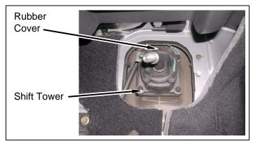
h. Remove four Torx bolts from shift tower mounting plate.
