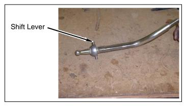
e. Install two plastic shift tabs, plastic ball, shim, and mounting plate onto shift lever.
