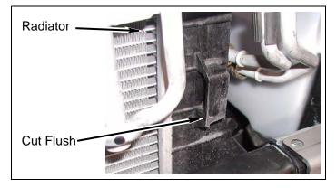
c. Install *kit* **bracket** (cooler, driver) and *kit* **bracket** (cooler, passenger) onto radiator with two bolts.
