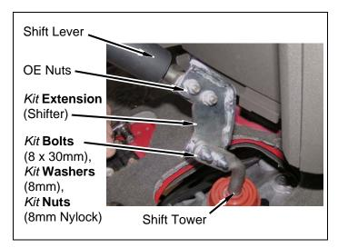
b. Install manual transmission shift lever onto *kit* **extension** (shifter) with two OE nuts.
