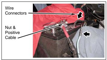
b. Install *kit* **bracket** (positive cable) onto passenger side positive battery cable with nut.
