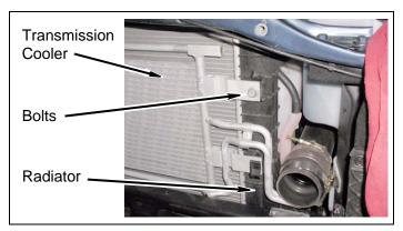
b. Carefully lift transmission cooler from radiator locking tabs.
