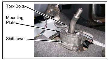
g. Install rubber cover onto shift tower.
