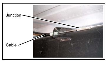
c. Remove front parking brake cable from driver side parking brake cable mount.
