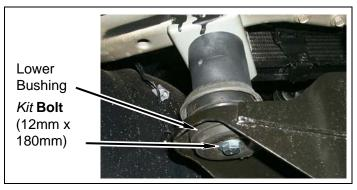
f. **2006 Models:** Install *kit* **bolt** (12mm x 180mm) into each cab mount. DO NOT TIGHTEN.
