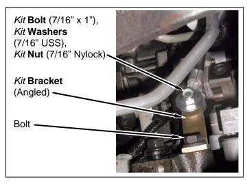
c. Install negative battery cable onto kit bracket (angled) with kit bolt (7/16" x 1"), two kit washers (7/16" USS), and kit nut (7/16" Nylock). TIGHTEN all hardware.
