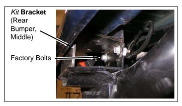
Apply small amount of kit Loctite® onto threads of factory bolts. Install two kit brackets (rear bumper) onto frame with four factory bolts. DO NOT TIGHTEN.
