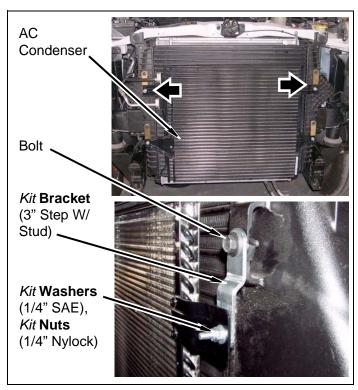
b. Cut excess threads from two *kit* **brackets** (3" step w/ stud).
