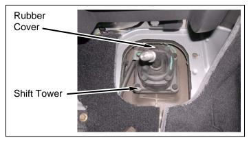
h. Install shift lever boot seal onto floor with six bolts.
