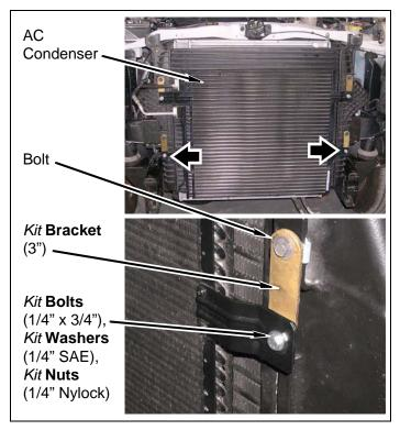
d. Install two *kit* **brackets** (3" step w/ stud), two *kit* **brackets** (3"), and AC condenser onto intercooler with four bolts. DO NOT TIGHTEN.
