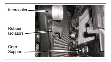
b. Install intercooler onto upper core support with two bolts.
