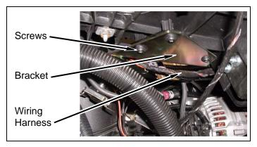
m. Install *kit* **bracket** (solenoid) underneath battery box with three screws.
