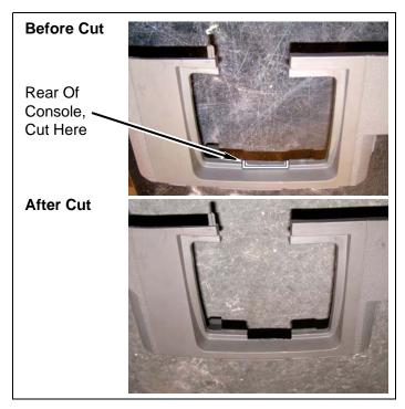
f. Install shifter console onto floor with two screws.
