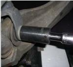
Install ReadyLift® SST kit onto strut using the factory hardware. Reinstall the strut into the truck. Apply pressure with a floor jack under the lower control arm near the ball joint to reattach the upper ball joint. Reattach upper sway bar end link. Be sure to torque all bolts to factory specs.
