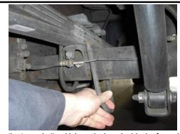
Remove the two u-bolts. Using a jack and a block of wood, carefully raise the truck by the leaf spring until the OEM block is loose and there is enough room for the new block.
