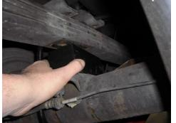
Install the ReadyLift® 2" rear block with the small taper facing forward. Lower the jack and make sure that the leaf spring center pin goes into the hole on top of the block.
