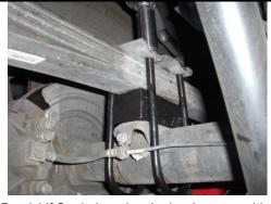
Install ReadyLift® u-bolts using the hardware provided. Torque to 120 ft/lbs. Repeat on opposite side.
