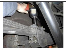
**REAR BLOCK INSTALLATION**Remove the four 21mm nuts.
