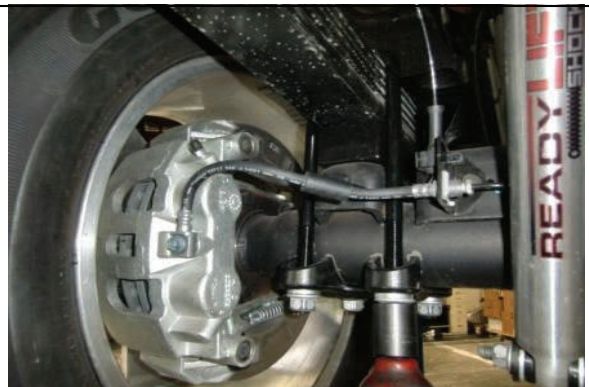
Torque U-bolts with vehicle on ground and re-clip ABS wire
