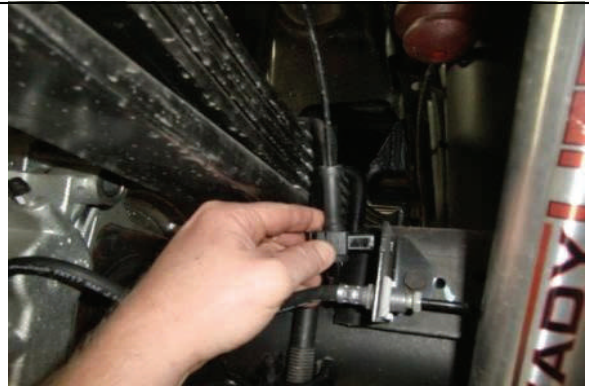
Release ABS clip from bracket on axle.
