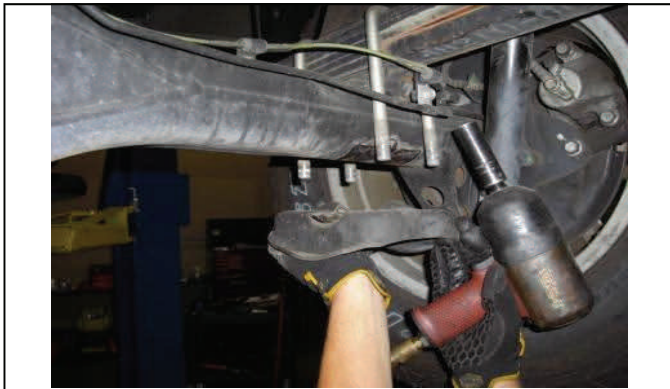
Remove u-bolt nuts and lower plate.
