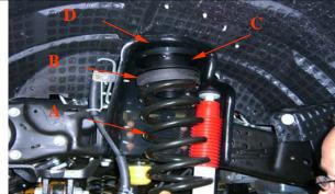
Install shock extension onto shock using the hardware provided. Please note that there is a driver and passenger side shock extension. Look for the D and P stamped on the inside leg of the brackets. Install shock extension bracket into factory shock mounting location on the axle using the factory hardware. Torque to factory specs.
