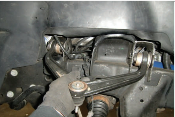
Remove upper control arm from frame pockets
