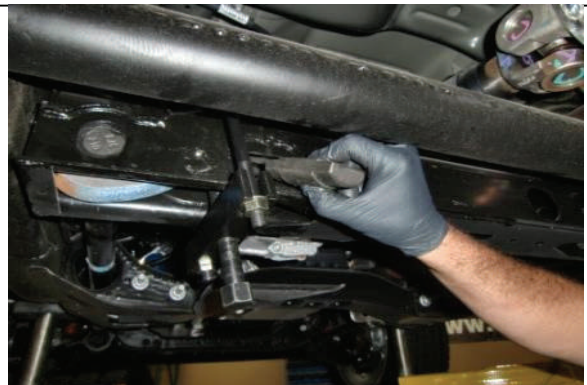
Adjust tool just enough to remove keeper block
