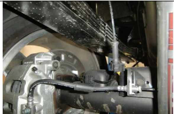
Carefully lower axle enough to install lift block
