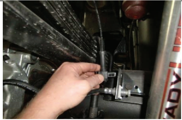
Unhook ABS wire from axle to prevent damage
