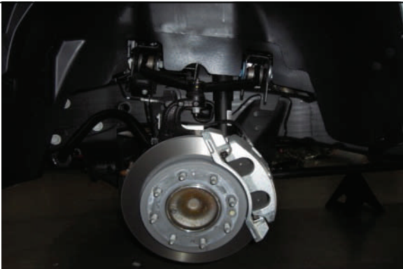
Securely lift vehicle and remove wheels
