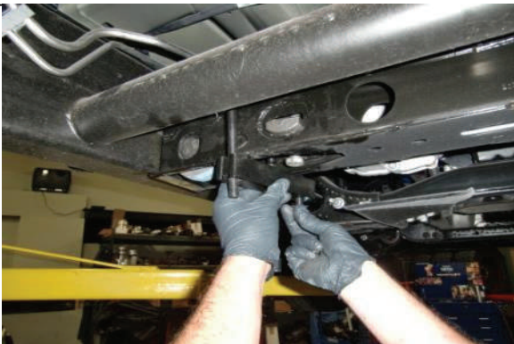
Position torsion bar unloading tool over cross member
