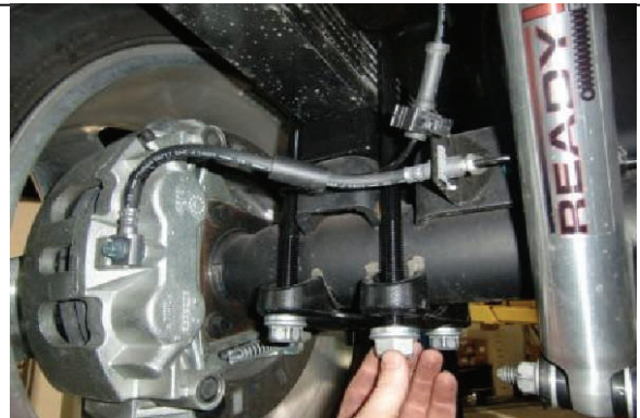
Install new longer u-bolts and install new hardware,
