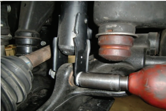
Loosen and remove lower shock hardware. New shocks req'd
