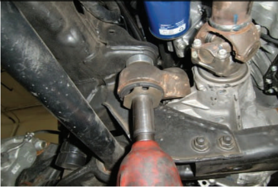
Install (4) differential drop spacers with new hardware
