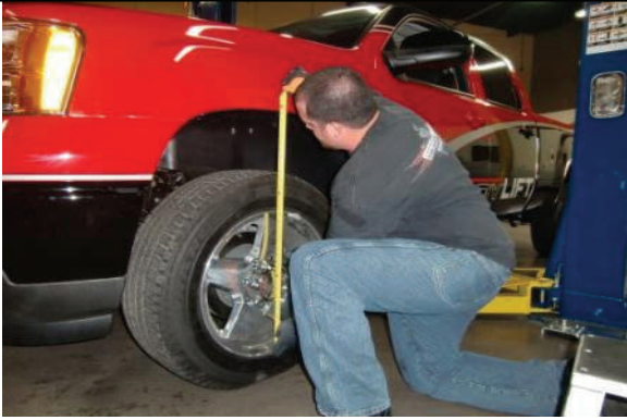
Measure ride height then lift vehicle and remove wheels/tires.
