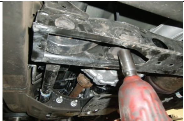
Remove torsion bar adjuster bolt. It will be reused.
