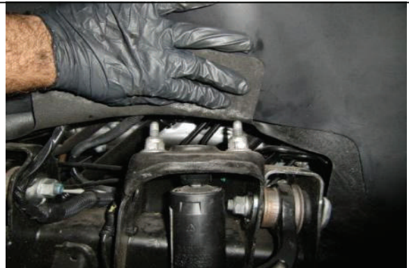
Push back soft fender liner to remove upper shock nuts.
