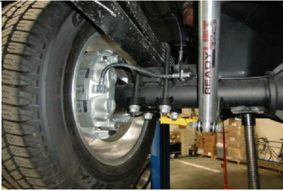
Properly support rear axle and disconnect lower shock mount
