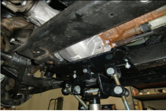
Support differential and remove differential mounting bolts
