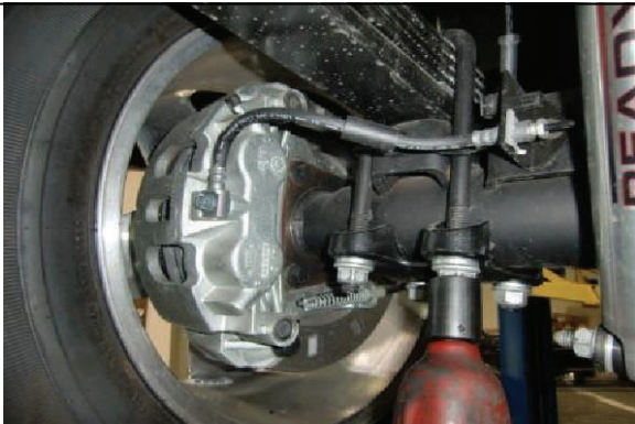
Loosen and remove u-bolt hardware
