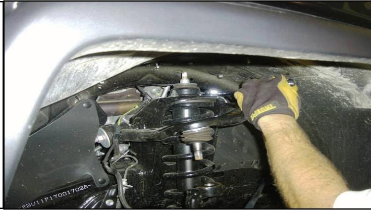
6. Remove the strut from the vehicle and mount it in a bench vise. Install the ReadyLift® kit, and torque fasteners to OEM specifications.
