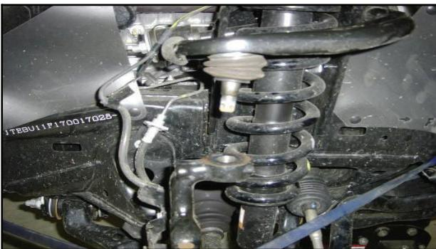
3. Remove ABS bracket bolts on the knuckle and upper a-arm.
