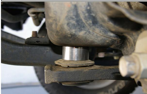
**11.** Install the 1" spacers between the differential supports and the front cross-member. Install the new bolts with factory washers and the new nuts and washers. Torque to factory specs.
