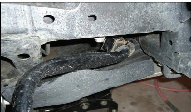
1. Starting from the passenger side, remove the sway bar end link nuts on both sides of truck.
