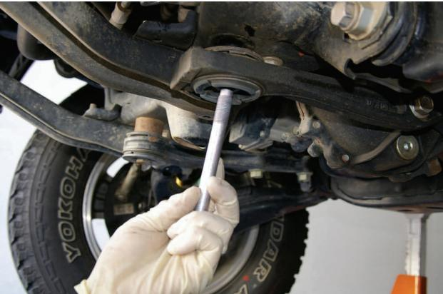
**10.** Remove the factory 19mm differential mounting nuts and bolts. The OEM washers will be reused.
