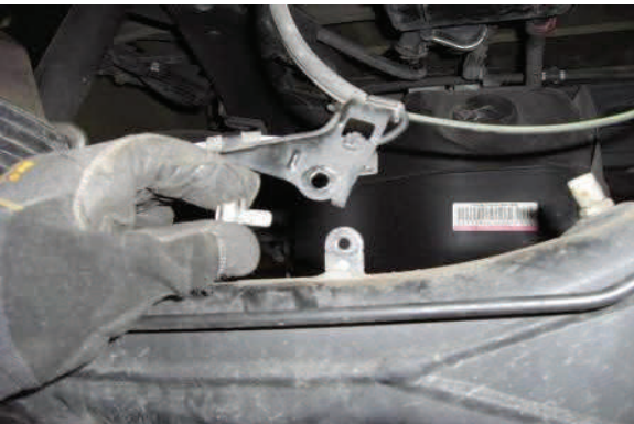
Disconnect ABS wiring brackets from axle.
