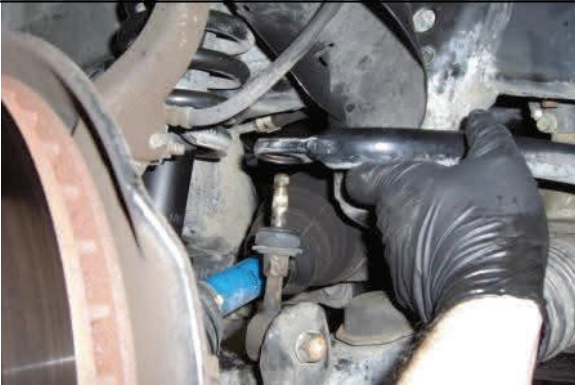
Shows earlier model sway bar end links
