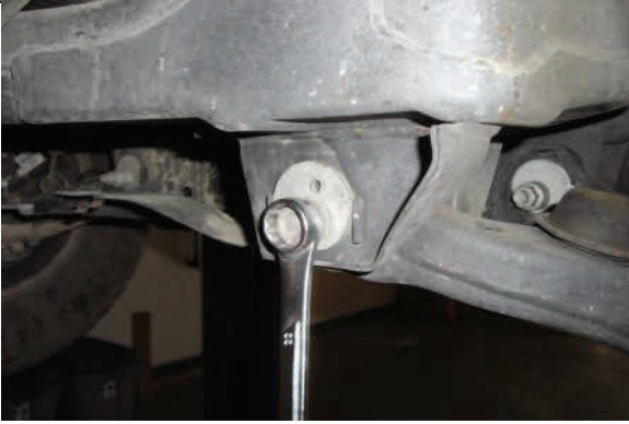
Mark and loosen lower control arm bolts, do not remove
