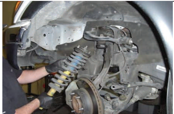
Remove strut from vehicle
