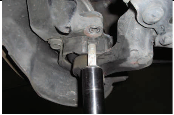
Disconnect lower ball joint hardware bolts
