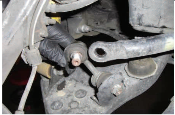
Disconnect dr./pass. side sway bar end links
