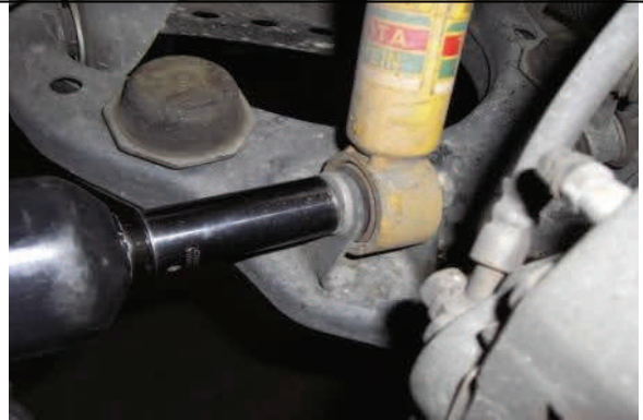
Disconnect lower strut mounting hardware
