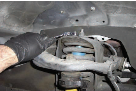
Disconnect upper strut mounting hardware
