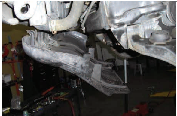
4WD models and 2.5-3.0" kits remove front skid plate
