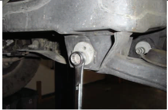
Reset and tighten lower control arm bolts
