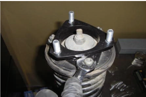
Attach new strut extension with OE hardware
