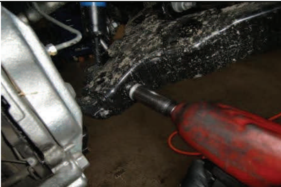
Reattach and tighten lower strut mounting hardware
