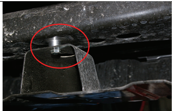
Install (2) skid plate spacers with new hardware
