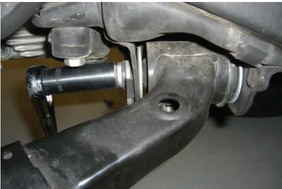
Loosen both lower control arm pivot/alignment bolts
