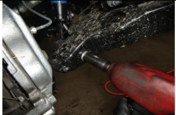
.Remove lower strut mounting hardware
