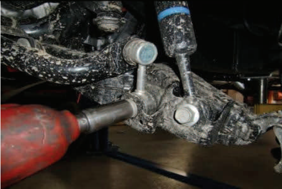
Disconnect lower sway bar end links
