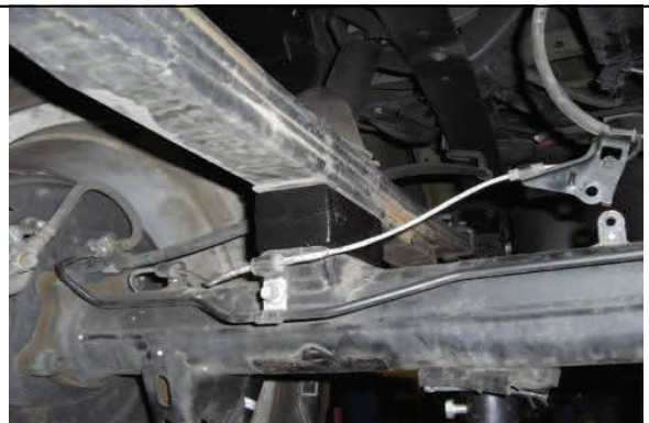
Raise axle and ensure locating pins are properly aligned.
