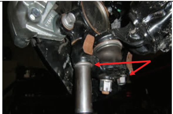
Remove (2) lower ball joint mounting bolts
