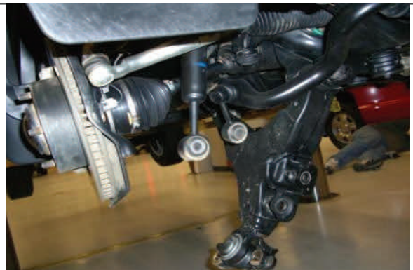
Swing down lower control arm and remove strut
