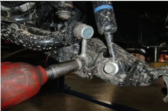
Reinstall wheels/tires, lower vehicle, reattach sway bar ends
