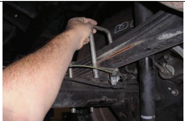
Carefully lower axle and remove u-bolts
