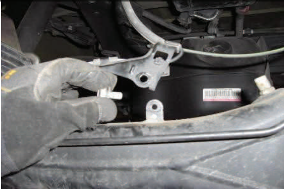
Disconnect ABS wiring brackets from axle.
