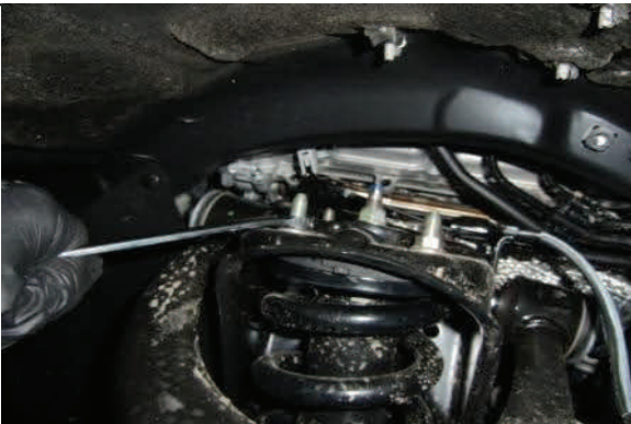
Remove upper strut mounting hardware
