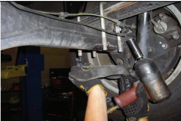
Remove u-bolt nuts and lower plate.
