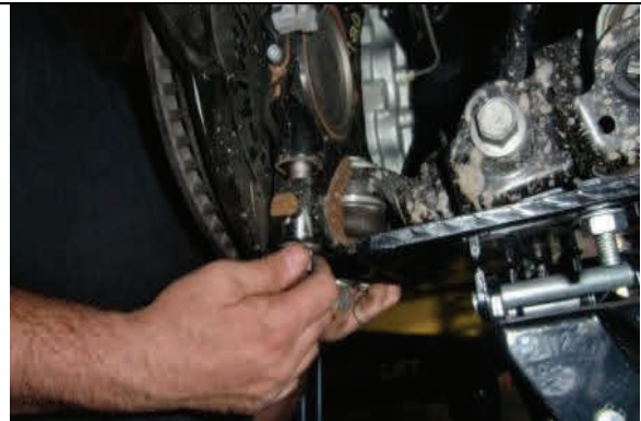
Raise lower control arm, reattach (2) ball joint mounting bolts
