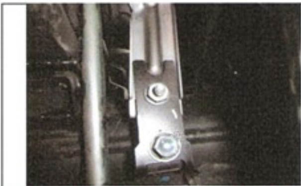
Install provided brackets with OE and provided hardware.
