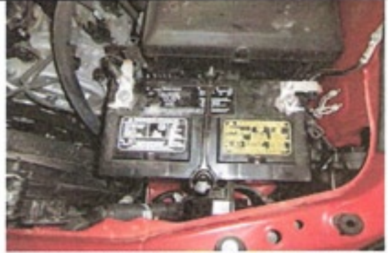
Disconnect positive/negative terminals and hold down clamp.
