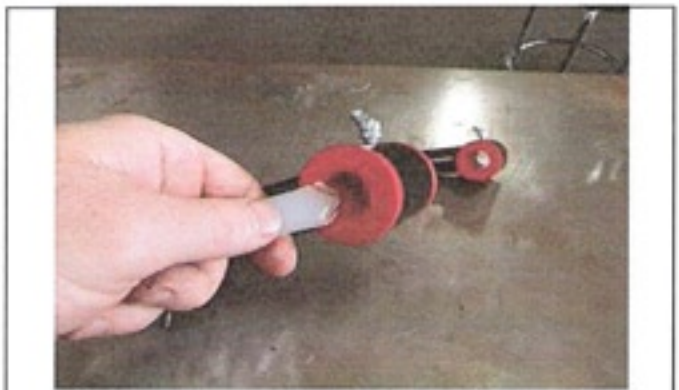
Apply grease to bushing center
