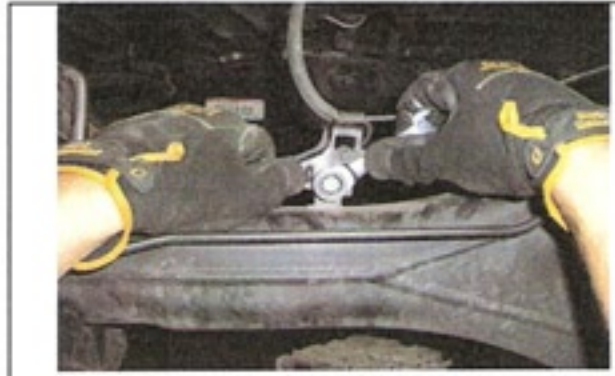
Replace shock on mount and ABS line to axle.
