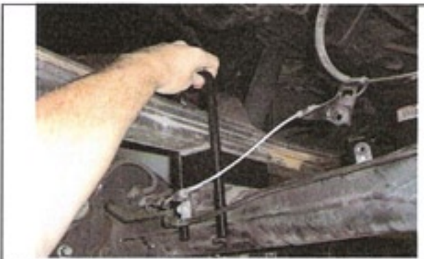
Slide new u-bolts over leaf pack and bump stop bracket.
