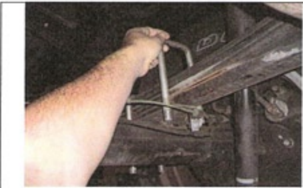
Carefully lower axle and remove u-bolts
