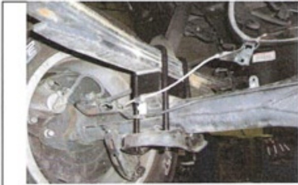
Attach lower mounting plate with provided hardware.
