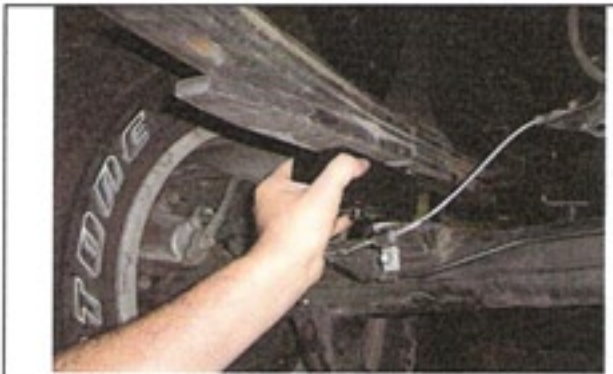
Place new lift block into position between axle and leaf pack.
