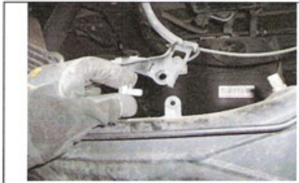
Disconnect ABS wiring brackets from axle.
