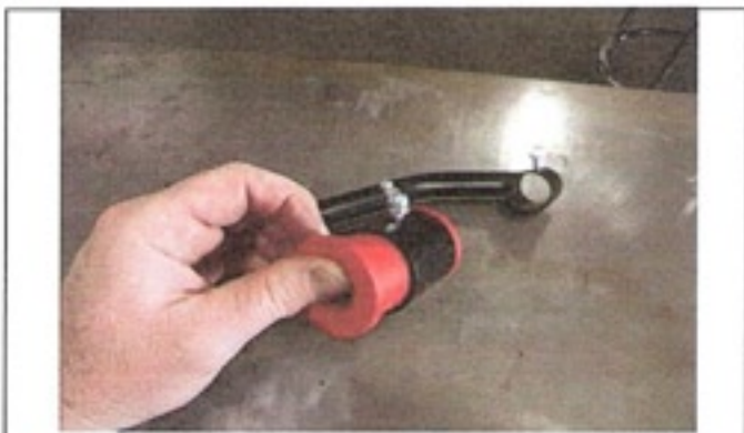
Install supplied retro bushings
