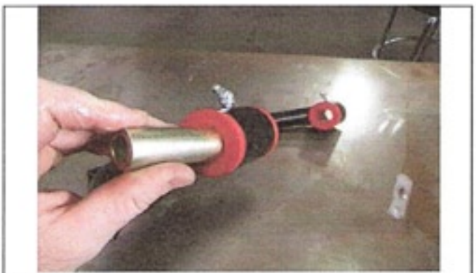
Install new crush sleeves into bushings. Wash hands!
