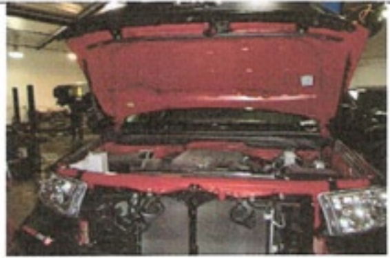
Raise hood to access battery and hose clamps on frame.
