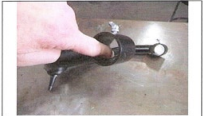
Evenly coat inner walls of both tubes
