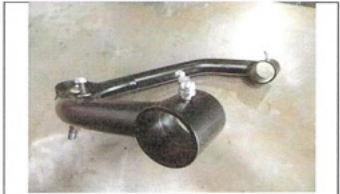
Remove old sleeves/bushings and clean pivot tubes
