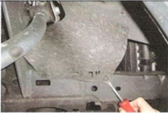
Remove slash guards at frame in front of upper control arms
