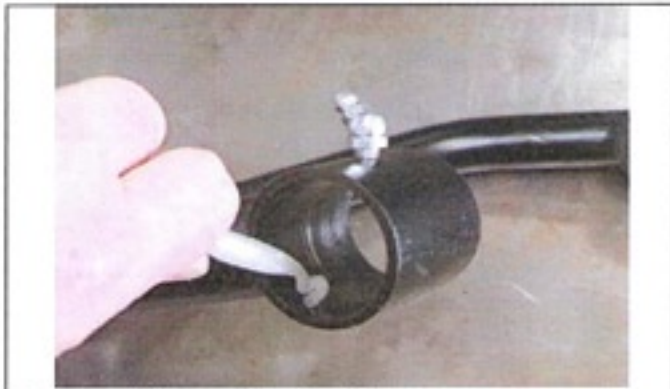
Apply supplied grease into pivot tubes
