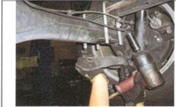
Remove u-bolt nuts and lower plate.
