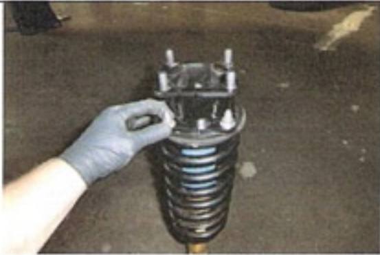
Install new upper strut spacer with OE hardware and torque.
