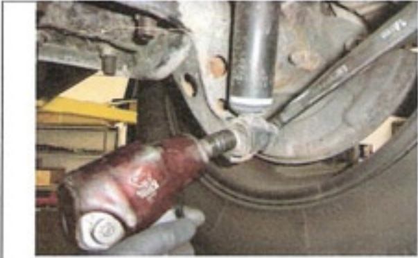
Remove rear lower shock bolt and disconnect shock.
