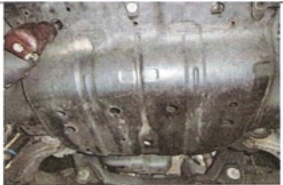
Remove front skid plate to expose sway bar.
