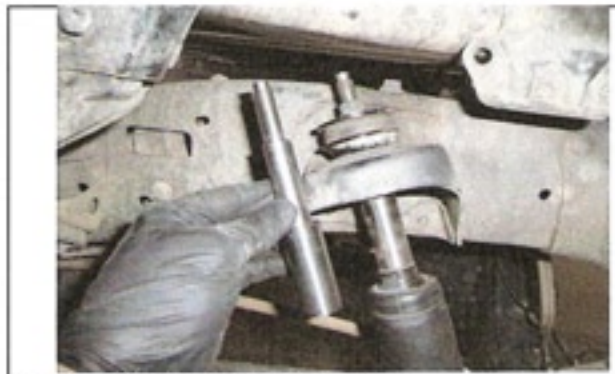
Install provided upper shock extension as shown.
