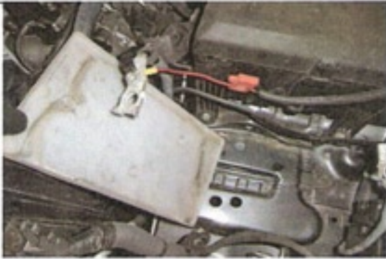
Remove battery and plastic tray from truck .
