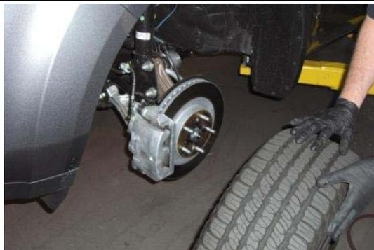
1. Open the hood and set at highest setting. Remove the front wheels. Starting on the driver side.
