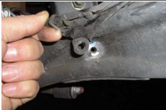
Remove the two 10mm bolts that hold the ABS line support
