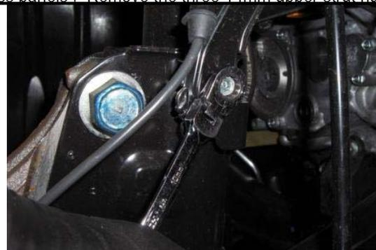
4. Use a 10mm wrench and remove the ABS line support bracket bolt.
