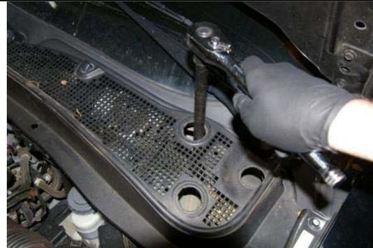
Tighten the three upper strut mounting nuts (14mm) 30 lb-ft.
