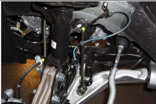
Install the supplied sway bar end link. Tighten to 85 lb-ft. Reinstall the brake line support bracket and ABS line support bracket using the OEM hardware.
