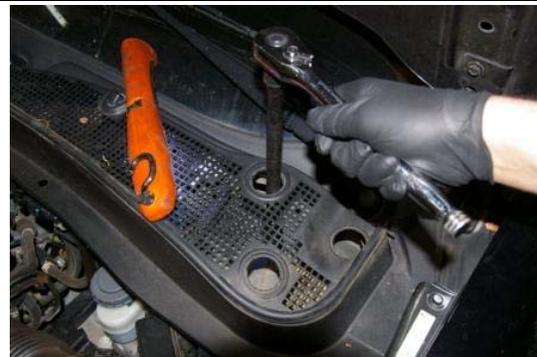
2. Use a flat screwdriver to remove windshield wiper access panels. Remove the three 14mm upper strut nuts.
