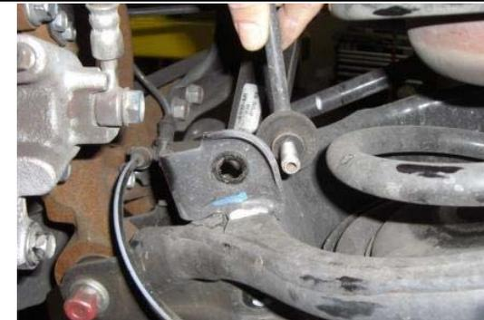
Unbolt the lower sway bar end link with a 14mm socket.
