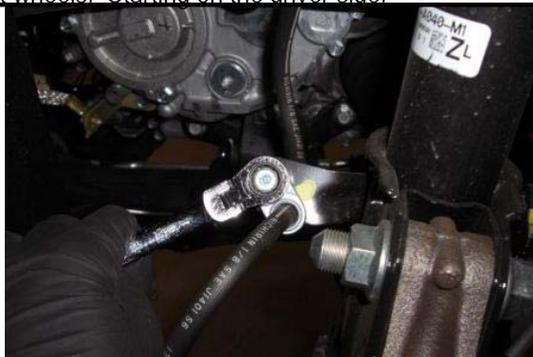
3. Remove the brake line support bracket using a 12mm wrench.
