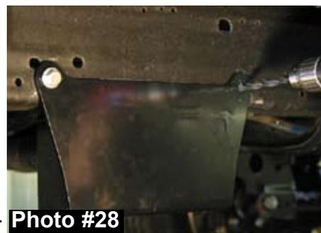
35. Locate the upper portion of the skid plate where it contacts the the frame. With all other bolts tight, mark and drill the three upper holes using 5/16 drill bit. Install the 3/8" thread cutter bolts. (See Photo #31)
