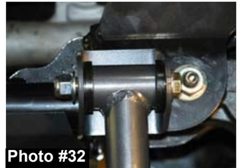
37. With the front bolts tight, install the bushings and sleeves into the rear of the strut bar. Attach the bracket to the bar using the same 1/2 x 4 bolt. Please note that the longer bracket is for the passenger side. With bracket attached to the rear of the strut bar, hold it up to the rear cross member. Mark the center mounting. Lower the bracket down and drill to 17/32. Once
