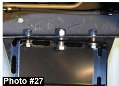
34. Attach skid plate to rear cross member and side braces using 3/8 x 1 fine thread bolts, washers, and self locking nuts. With all bolts started, tighten all bolts including the skid plate braces. (See Photo #30)
