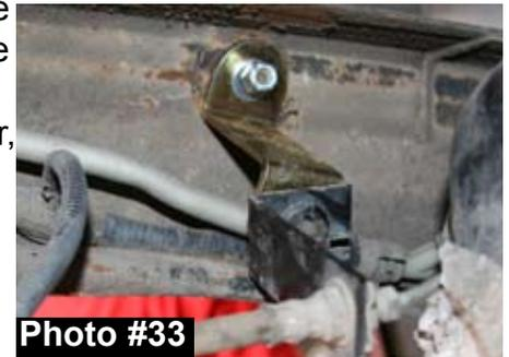
drilled reinstall using 1/2 x 1 1/2 fine thread bolt, washers, and lock nut.
