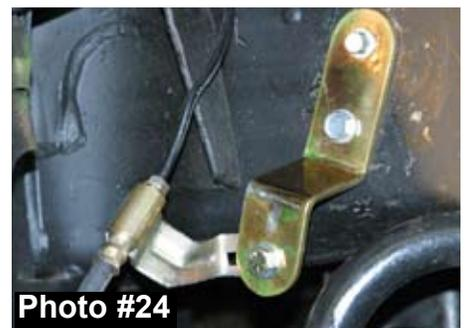
29. Install the new Skyjacker sway bar end link bushing (Part # SBE-CBSH) on the stud of the pivoting end of the new Skyjacker sway bar end link with the larger diameter end facing the boot of the sway bar end link. Align the sway bar end link bushing with the OEM mounting location of the OEM a-arm & install the new Skyjacker sway bar end link. Note: Be sure to install the sway bar end link with the pivoting end at the a-arm. (See Photo #25 and #26)
