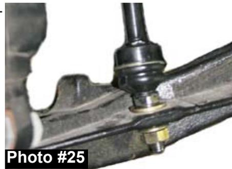
30. Install the new Skyjacker shocks using the factory bolts on the bottom.
