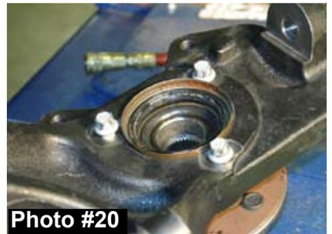
24. Install the new steering knuckle by attaching it to the upper and lower A - Arm ball joints.
