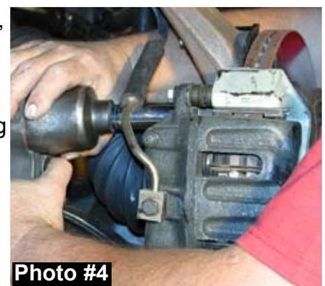
6. Remove the cotter pin from the axle shaft. Remove the axle nut using 1 7/16" socket. (See Photo #5)
