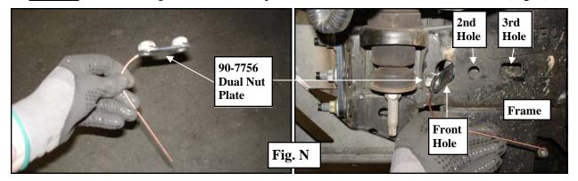
Step 17: Install the upper support plate (93-7608 Drvr and 93-7609 Pass) from the outside behind the core support, and secure the rear of the plate to the dual nut plate (90-7756) through 2nd & 3rd holes in the frame rails using the (2 per side) supplied 1/2" X 1 1/2" bolts and washers. Leave bolts loose at this time. (Fig O)
