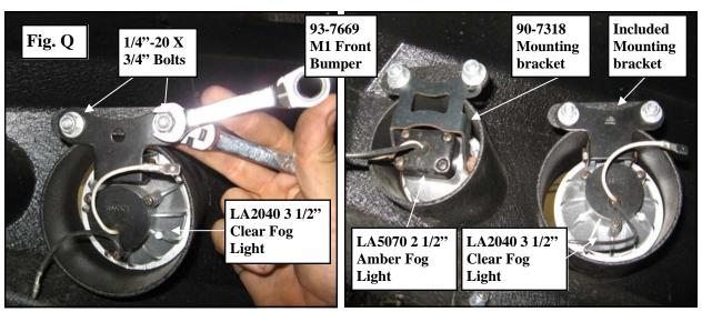
Step 23: Install the fog lights into the new M1 front bumper (93-7669) using the supplied (4 per side) 1/4"-20 X 3/4" bolt and hardware. (Fig Q)
