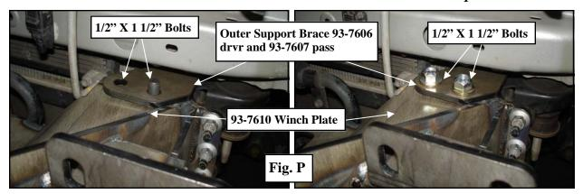
**Step 19:** Torque all of the **1/2**" winch plate and bracket assembly mounting hardware to **85** ft./lbs or **OE** hardware to manufacturers specifications.
