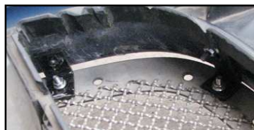
Figure 3 – Rear view of vehicle's shell; Grills attached with Metal Brackets and Flange Nuts
