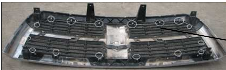
Figure 3 – Rear view of vehicle's shell; Grills attached with Metal Brackets and Flange Nuts
