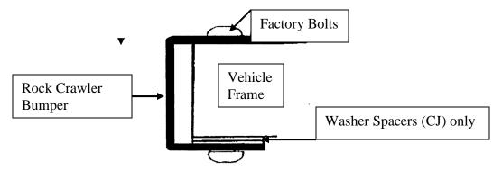
**Step 3:** Tighten all hardware at this time. Installation is now complete.
