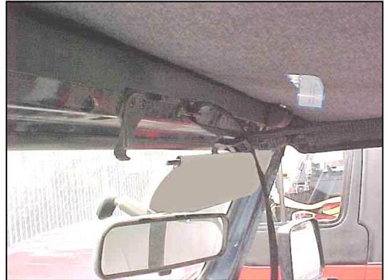
7. Re-adjust Velcro and tighten all straps to assure a wrinkle-free fit.
