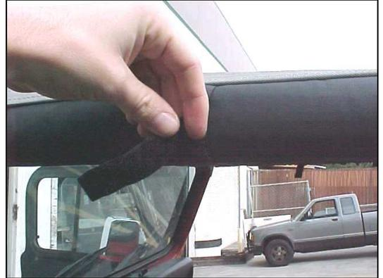
6. Locate the center strap along the central roll bar. Run the center strap around the rear and under the central roll bar forward to the Footman Loop near the top center of the windshield. Run strap through Footman Loop and feed strap through its buckle securely (Figure 9).
