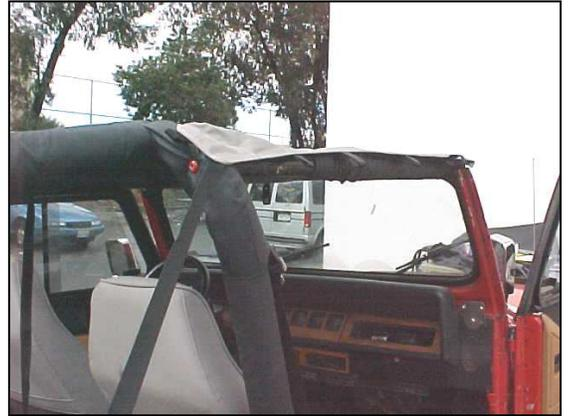
4. Pull the straps under the central roll bar through the Side Loops #1, then pull the straps towards the rear of the vehicle and insert through the Rear Loops #2 (Figures 5 & 6). Attach the strap to the mating buckle #3 (Figures 6 & 7).
