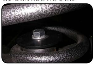
16. Install new rear sway bar links on the inside of the sway bar and the inside of the axle bracket. Use the factory bolt on the axle side with the nut on the outside so excess threads will not interfere with the shock. Use the provided 12mm bolt and washer for the top side with the 12mm nut and washer on the inside to give the most possible room for tire clearance. Torque to 75 ft-lbs.
