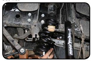
30. Install the new sway bar links, on the outside of the sway bar and inside of the axle mount. Torque to 75 ft-lbs.
