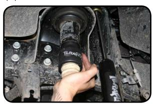
29. Install new 3 inch coil springs. Do the drivers side first.
