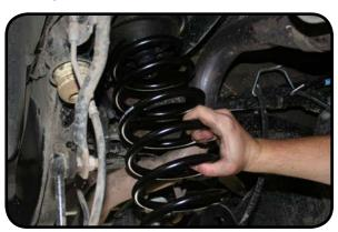
12. Use grease and install new upper spring guide spacer by popping it into the factory location.
