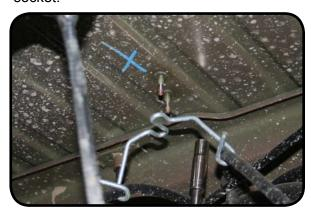
11. Carefully lower the rear axle far enough to remove the rear springs. Be careful not to let the coils fall out as you lower the axle. You will want to lower the axle far enough to install the new 3" springs in place. While lowering the axle make sure the brake lines, ABS wires and axle vent do not stretch as this could cause damage to these vital parts.
