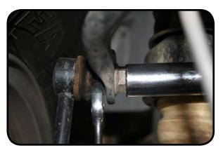
8. Remove the clips that secure the ABS wiring harness to the upper control arm mount.
