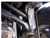
22.Place the brace with the fixed end in the factory trackbar bracket and the bend upward. Use the 9/16" bolt to hold it in place. Do not tighten at this point.
