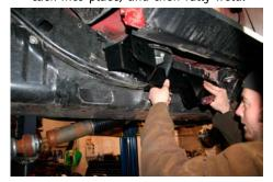
On the driver side hold the bracket into place. There is no hole to match up the to on the frame so the exact location should be determined by measuring the other side and matching the driver side to it. Mark the bracket and the frame for welding preparation. Remove the bracket and clean off the paint from the bracket and the frame
