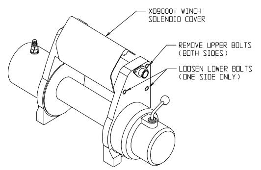
• If the winch has a separate control pack with a black plastic cover, remove the plastic cover being careful not to strain the internal wiring. Replace the cables as described above. Reinstall the cover.
