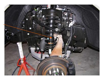
13. Reinstall the brake line bracket to the strut tower.
