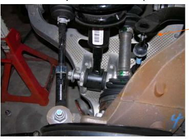
4. Disconnect the brake line from the strut tower.
