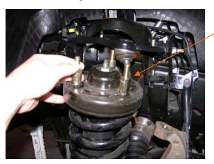
9. Install the spacer lift on top of the strut plate.
