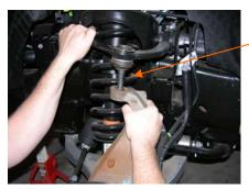
6. Remove the 3 upper strut mounting nuts on the top off the strut tower.
