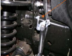
5. Separate the upper ball joint from the spindle. Use a ball joint separator or other suitable tool.
