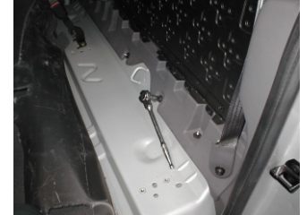
Remove rear panel bolts.
