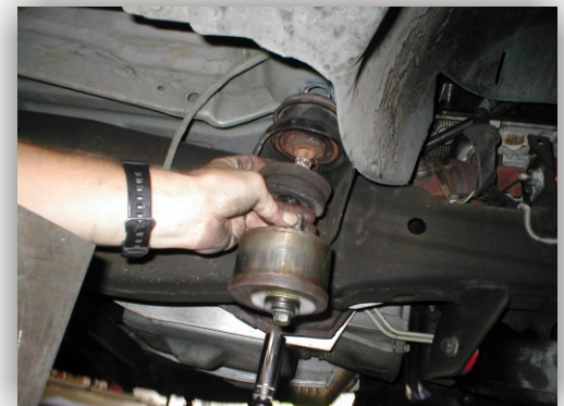
Remove body mounts
