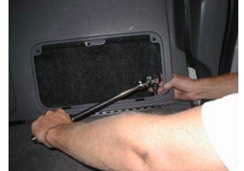
Flex out panel to access bolt.
