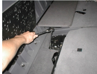
Remove rear seat bolts.
