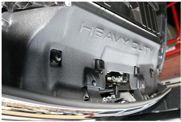
A. Remove the OEM lower air Dam by popping out the plastic clips.
