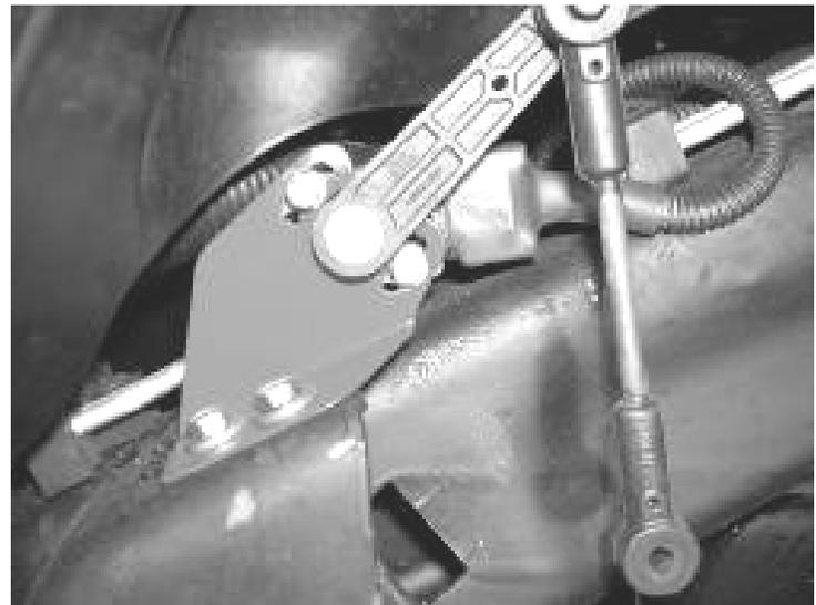
67. Install the FT20098 brake line extension tab using the original bolt and the supplied 5/16" hardware. **SEE PHOTO IN NEXT COLUMN.**
