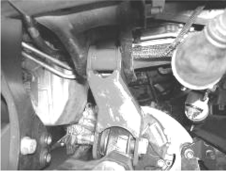
24. Place the differential housing into the Fabtech rear crossmember using the supplied  $\frac{1}{2}$ " x  $4\frac{1}{2}$ " bolt, nut, and washers along with the supplied large FT55-1 washers attach the differential. SEE PHOTO ON NEXT PAGE.
