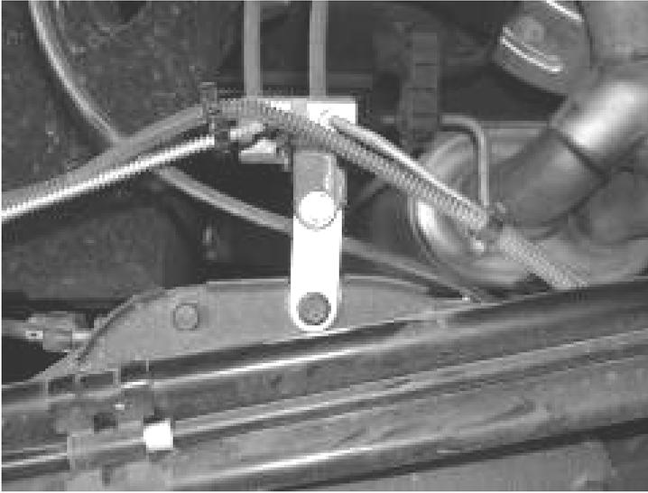
68. Raise the floor jack supporting the rear axle and slide the lower mount of the track bar into the new bracket on the axle. Torque to 105ft. lbs. SEE DIAGRAM BELOW.
