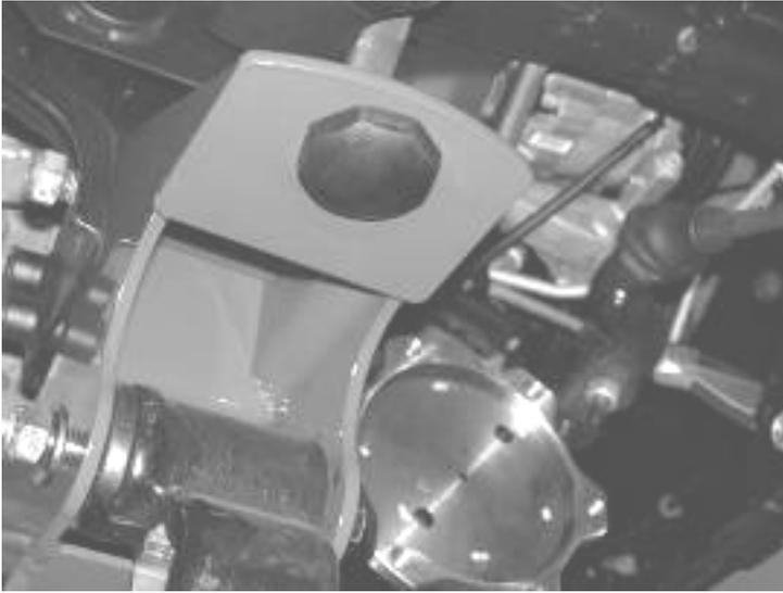
31. Locate the factory brake line mount on top of the upper control arm. Remove the brake line mount, and route the line with bracket to the bottom side of the control arm. Drill a guild hole directly below the original hole on the upper control arm. Mount the factory bracket to the bottom side of the control arm using the supplied 5/16 thread forming bolt. SEE PHOTO BELOW.
