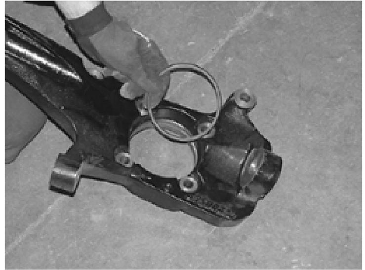
33. Working from the driver side of the truck, attach the steering knuckle FT20246D for the driver side to the upper control arm and to the lower control arm using the stock hardware. Torque the upper ball joint to 35 ft lbs and lower to 70 ft lbs.
