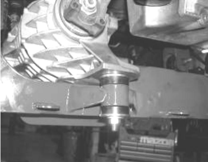
25. Locate and insert the square FT20058 tab bolts into the stock front control arm crossmember and through the holes outboard of the removed stock splash shield mounting holes. Attach the Fabtech front crossmember into the lower control arm pockets using the stock hardware. Use the  $\frac{3}{8}$ " nuts and washers from hardware kit to attach the tab bolts to the under side of the crossmember. Leave loose. SEE PHOTO BELOW.
