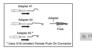
Connect adapter to "HOT" side of the fuse. With the ignition on, the compressor will turn on and fill the system to 10 p.s.i. before shutting off.
