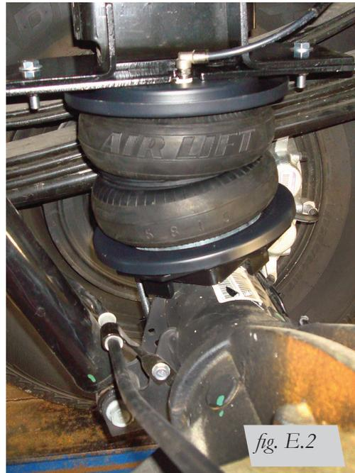
Inside view of the passenger's (right) side installation.
