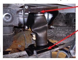
Make sure the fitting and thread post go through the slot in the upper bracket.
