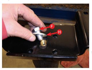
Loosely attach the spring (C) to the lower bracket (B) with the 1/2" bolt (F) and flat washer (H).
