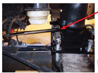
Raise the inside of the lower bracket up enough to slip a 3/4" wrench over the 1/2" bolt and torque to no more than 15 ft-lbs.
