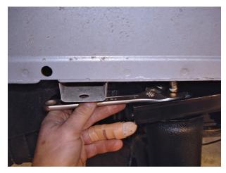
Adjust air spring and torque to no more than 4 ft-lbs. using a medium size crescent wrench or open end wrench.
