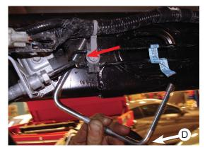
Figure 4 shows U-bolt (D) being installed on the inside of the left (driver-side) frame section on the back side of the jounce bumper mounting location.
