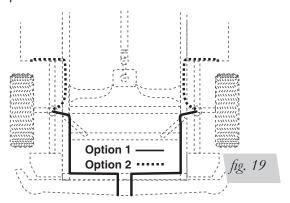
7. Cut off the air line, leaving approximately 12" of extra air line. A clean square cut will ensure that the line will not leak. Insert the air line into the air fitting. This is a push-to-connect fitting. Simply push the air line into the 90° swivel fitting until it bottoms out (9/16" of air line should be in the fitting).
