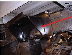
Figure 8 shows the left (driverside) outside frame with the upper bracket over the U-bolts and in position.
