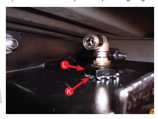
Set 3/4" serrated flat washer (K) over fitting and thread post on the air spring. Thread the nylon jam nut (L) onto the thread post. Torque to finger-tight only.
