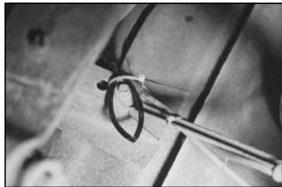
A kink or fold in the air line. Re-route as needed.
